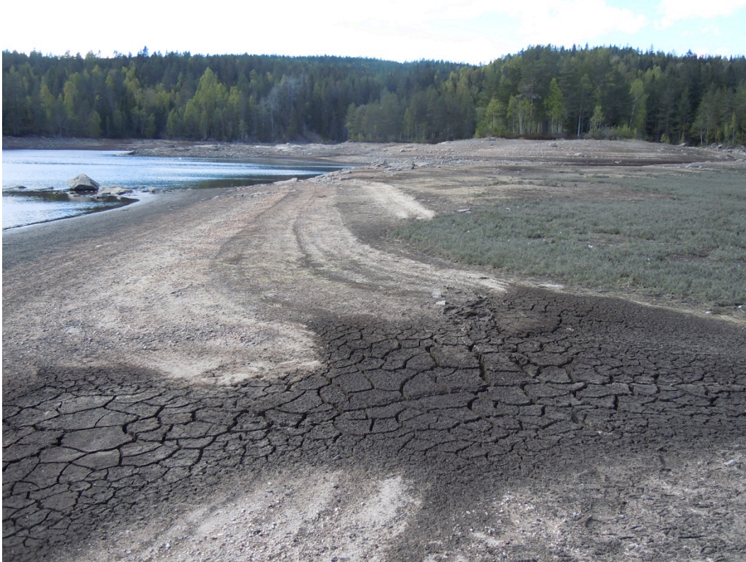
Photo 1. Erosion of the silty-clay layer depending on the intensity of waves during lowering the water level. 19.05.2020.
